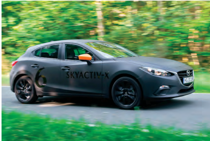
The next-generation Mazda3 (left) will debut the SkyActiv-X engine, which uses spark-controlled compression ignition to provide the most efficient aspects of both diesel and gasoline engines, generating up to 20 percent better fuel efficiency. The 2019 Infiniti QX50 (right) dropped its fuel consumption by 27 percent compared with the current model, in part by deploying a turbocharged, downsized engine with a variable compression ratio.
