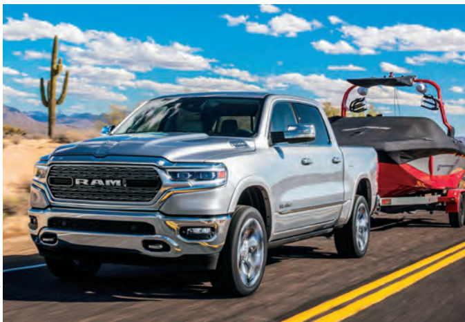
The 2019 Ram 1500 comes with a 48V stop-start system that not only diminishes idle fuel use but also provides additional torque from an electric motor to supplement the engine at low speed.
