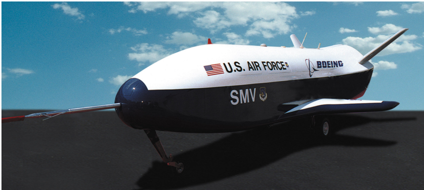
Figure 9.3. This photo shows the X-40a, a 6.7 m long model of an SMV built for testing.
