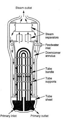
As implied by its name, the function of a steam generator is to produce steam. Hot water from the reactor vessel enters the tubes via the primary inlet and exits through the primary outlet shown in Figure 7. Water is supplied to the area outside the tubes through the feedwater inlet. Baffles force this feedwater flow to first encounter the tubes at their lower regions. The feedwater is heated to the boiling point as it flows upward along the tubes.
