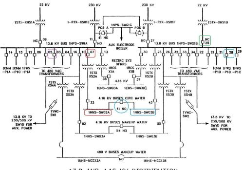
Figure 4 Electrical distribution system at River Bend
