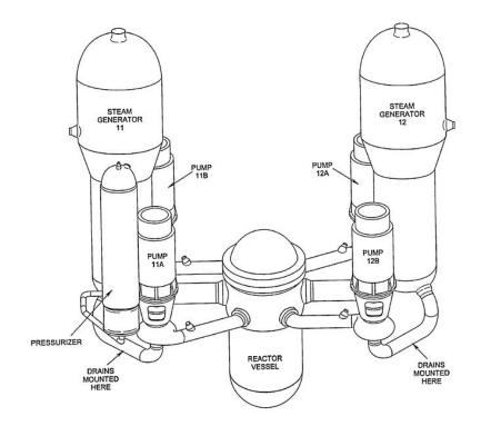
Figure 5: Primary system components at San Onofre
