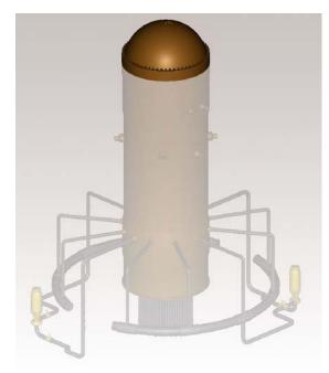
Figure 2: Reactor vessel and its head
