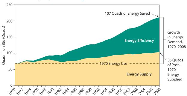
FIGURE 4.2. Efficiency Helps Meet U.S. Energy Demand
