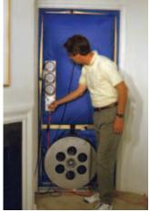
A blower-door test finds leaks A properly sized HVAC that can be sealed, creating an airtight building with minimal heat and air-conditioning loss.
