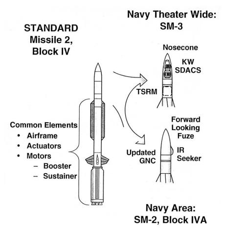
Figure 1: A comparison of the SM-2 Block IV, Block IVA, and SM-3 missiles.
