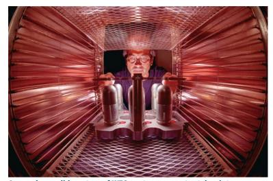
An employee slides a tray of W76 neutron generator tubes into a desiccator (drying) cabinet at the Explosive Components Facility at Sandia National Laboratory.
