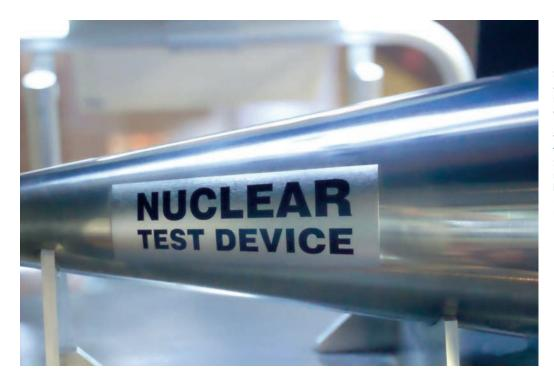
Scale model of a nuclear weapon resting on a diagnostic rack or "jewel rack" used for weapons testing at the Nevada National Security Site. The model was built by the Los Alamos National Laboratory, Los Alamos, NM.
