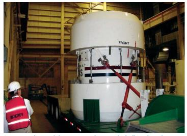
Storage cask containing transuranic waste including plutonium being put on a trailer at the Waste Isolation Pilot Plant (WIPP) in New Mexico, 2002.
