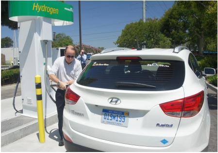
This fuel cell electric vehicle is being refueled with hydrogen produced from a sewage treatment facility. Biological sources of hydrogen result in much lower net global warming emissions than hydrogen produced from natural gas.
