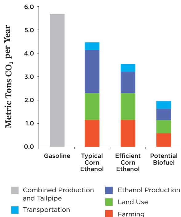
*While improvements have been made to ethanol production, the potential exists to reduce emissions throughout the entire lifecycle of biofuels. Emissions reduction strategies include using biogas from anaerobic digesters as a source of process heat and switching from corn to wastes, residues, or perennial grasses.*
