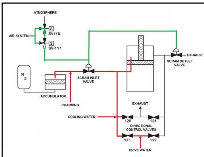
conditions. The directional control valves are normally closed, and they open when signals are sent to their electric motors.
