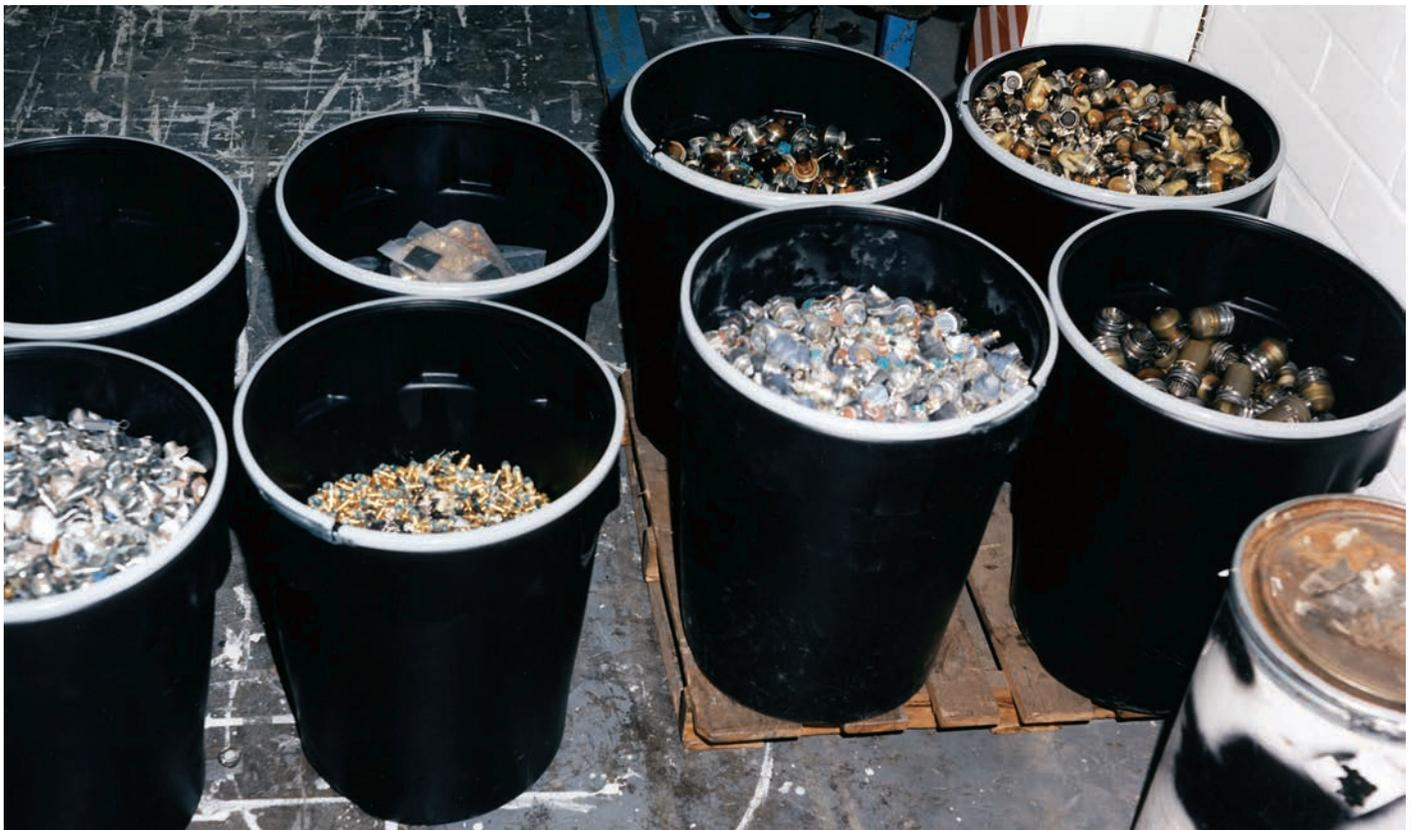
As part of the dismantlement of warheads at the Pantex plant in Texas, copper, aluminum, silver, gold, plutonium, and non-nuclear weapons parts are separated for recycling, 1992.
