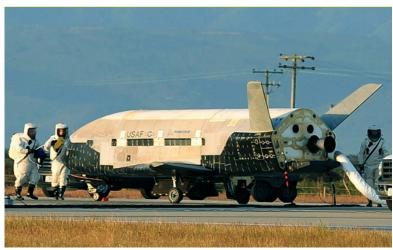
Technicians inspect an X-37B in June 2012 after it completed the program's second mission. Photo: USAF/Boeing
