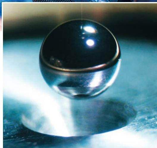
**A two-millimeter-diameter capsule filled with a deuterium-tritium (DT) gas, surrounded by an 80- to 100-micrometer-thick layer of DT ice, which is the target for the lasers of the National Ignition Facility.**
