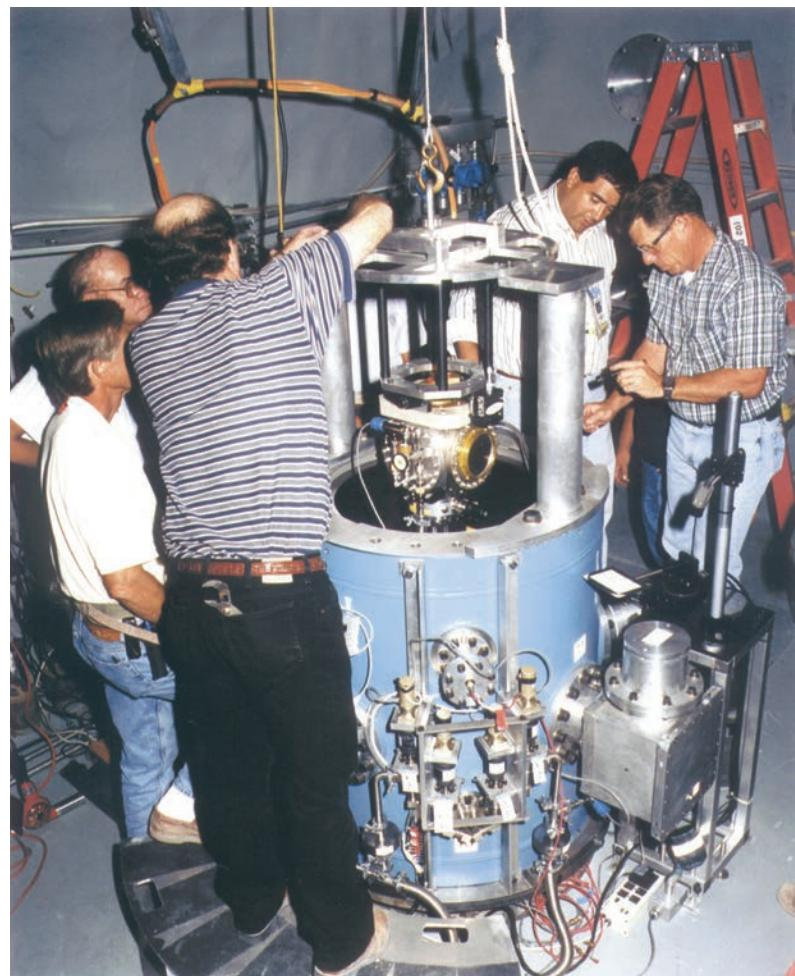
**Workers from Lawrence Livermore National Laboratory and the Nevada Test Site lower the “cube” containing plutonium and chemical explosives into the confinement vessel to conduct a subcritical experiment, 2000.**
