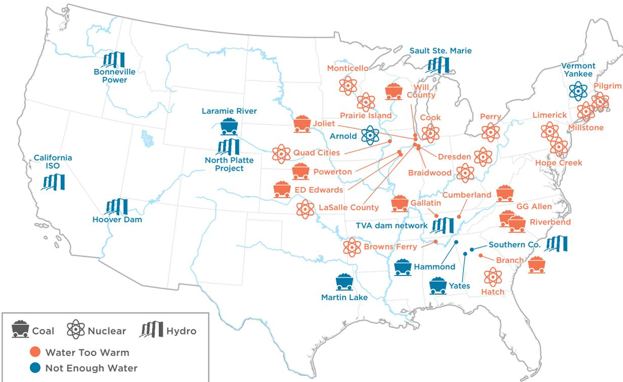
*When water used to condense steam at power plants is too hot or supplies shrink, the plants run into trouble. Operators have had to shut down or curtail production at numerous power plants because of water-related risks in recent years.*
