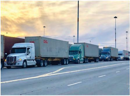
Semi trucks that transport cargo containers to and from ports and railyards ("drayage trucks") often travel short distances per trip and are well-suited for electrification. Several electric models, with ranges up to 300 miles, are already in demonstration today.
