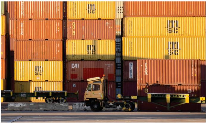
Four manufacturers already offer electric versions of yard trucks, which move cargo containers within port, railyard, and warehouse complexes.
