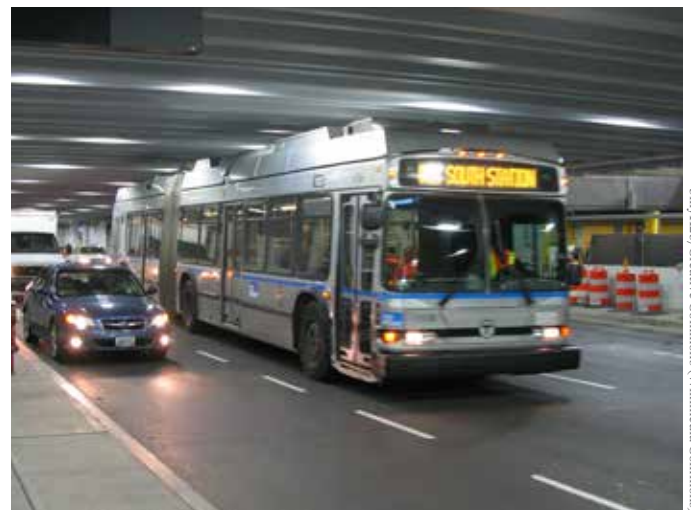
While ride-hailing can get cleaner by using electric vehicles, so can mass transit. This bus between downtown Boston and Logan Airport runs part of each trip on power from overhead electrical wires.
