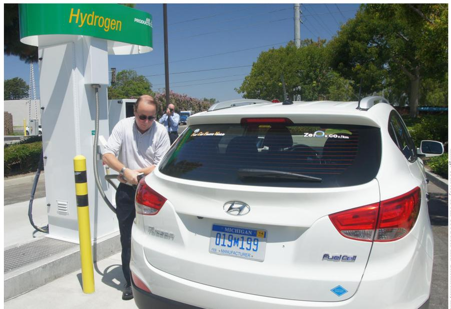
*This fuel cell electric vehicle is being refueled with hydrogen produced from a sewage treatment facility. Biological sources of hydrogen result in much lower net global warming emissions than hydrogen produced from natural gas.*
