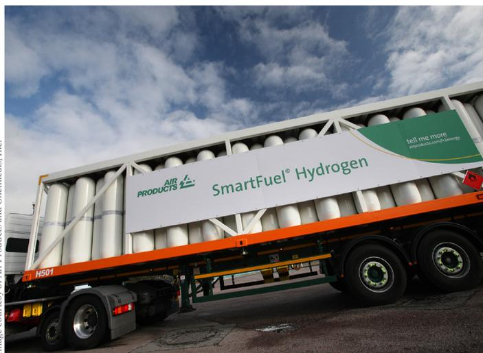
The hydrogen gas that powers fuel cell electric vehicles is often transported from a central production facility to refueling stations in high-pressure tube trucks like this. Centralized hydrogen production is generally more cost-effective than distributed (or local) production.
