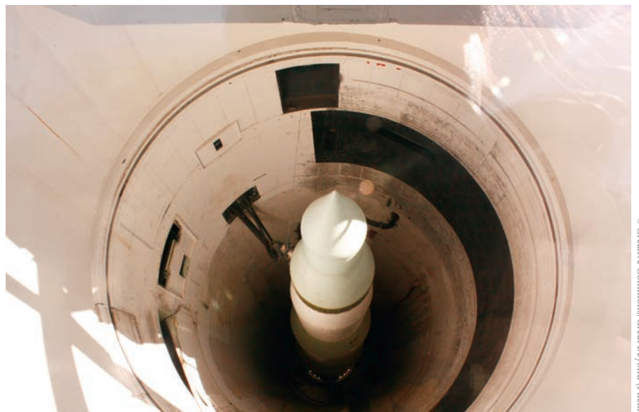
A Minuteman II missile in its silo. “Safing” missiles (using a switch that isolates the missile from outside launch signals) eliminates the risk of an accidental or unauthorized launch.
