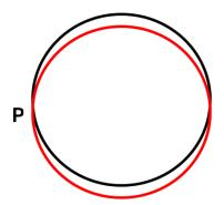
Figure 9: The orbital module follows the black orbit and the CompanionSat follows the red orbit. The orbits cross at point P and at a second point on the other side of the orbit.
