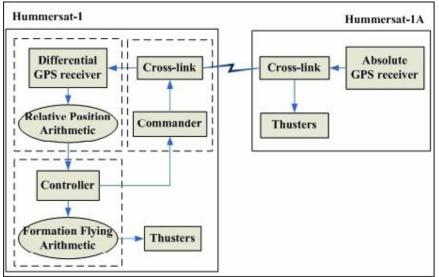
Figure 12: Guidance process for the HummerSats. (image credit: DFHSat)
