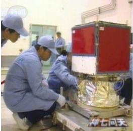
Figures 4: A photo of the Companion Satellite being prepared for launch. The solar panels are covered with protective sheets. (Image credit: CCTV,
