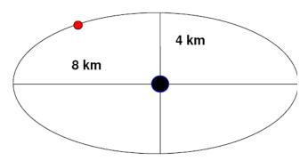
Figure 10: from the perspective of the orbital module (black dot), the CompanionSat (red dot) circles around it on an elongated orbit at a nearly constant speed of about 5 m/s.
