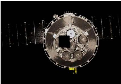
Figure 7: This picture of the top of the orbital module was taken by the CompanionSat 6 seconds after it was released on 27 Septebmer. The black square is the shadow of the satellite. In the background, the solar panels of the service module are visible (http://news.xinhuanet.com/english/2008-10/05/content\_10152706.htm).
