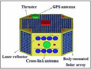
Figure 11: The HummerSat-1A. (image credit: DFHSat)
