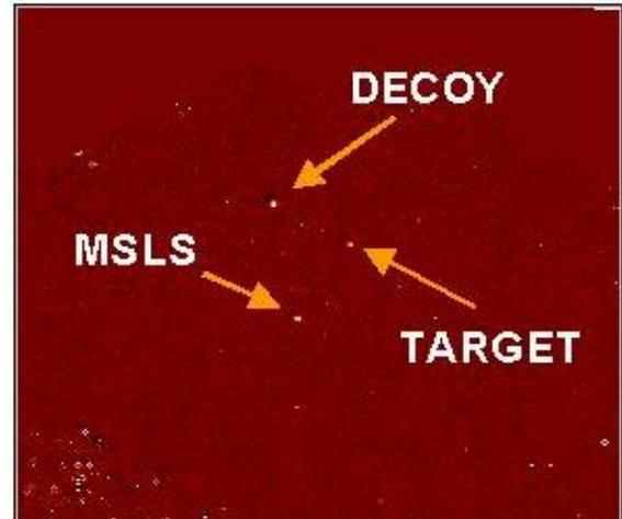
*Until about two seconds before impact, the objects simply appear as points of light to the kill vehicle. The kill vehicle is able to recognize each object based on stored information it has about the objects' brightness and fluctuation.*
