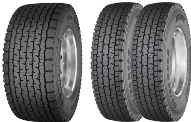
*Single-wide tires (left), which replace a traditional dual-tire configuration (right), not only weigh less but also can improve fuel efficiency by reducing the amount of energy lost to tires flexing during travel.*
