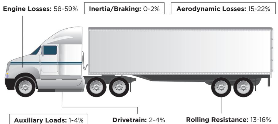
*At highway speeds, more than half of the energy contained in diesel fuel is lost to inefficiencies in the combustion process of the engine. The remaining energy is used to move the vehicle down the road and to operate auxiliary loads such as air conditioning, heating, and electronics.*
