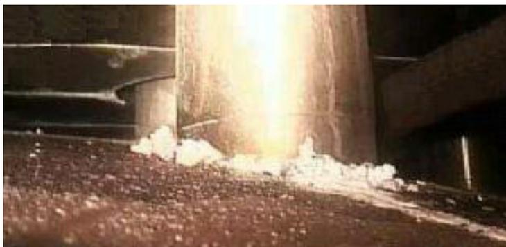
Boric acid crystals on the outer surface of a reactor vessel head at a plant similar to Davis-Besse.
