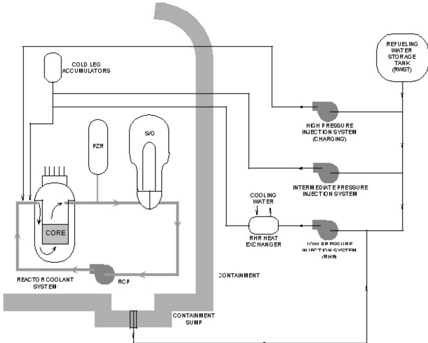
To compensate for the reactor water exiting through the hole, water inside the pressurizer (PZR) and the cold leg accumulators flows into the reactor vessel. This initial makeup is supplemented by water from the Refueling Water Storage Tank (RWST) delivered to the reactor vessel by the high, intermediate, and low pressure injection pumps. The makeup water re-fills the reactor vessel and overflows out the hole in the reactor vessel head.
