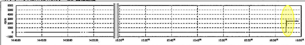
The two charts above show the RCIC system flow rate in liters per second (top) and the RCIC turbine speed in revolutions per minute (bottom).
