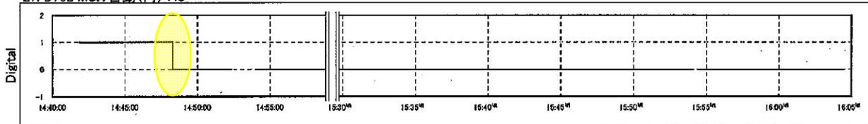
About a minute after the reactor shut down, the main steam isolation valves (MSIVs) closed. The chart above shows the logic signal for the MSIVs – a “1” indicates the MSIVs are open while “0” indicates the valves are closed. The alarm printouts are not available for Unit 2 as they were for Unit 1. It is assumed that the MSIVs closed on Unit 2 for the same reason they closed on Unit 1 – loss of normal power supplies when the turbine tripped.
