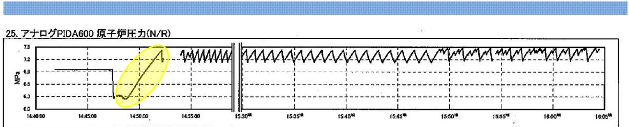
The closure of the MSIVs changed the trend of pressure inside the reactor vessel. Pressure had been trending downward as the amount of steam produced by the reactor core's decay heat was transported through the steam pipes to the turbine and condenser. When the MSIVs closed, the steam had no place to go. Bottled up inside the reactor vessel, the continued production of steam caused the reactor vessel pressure to steadily increase for the next five minutes.
