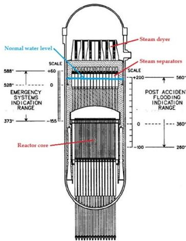
For this instrument, 0 mm corresponds to the bottom of the steam separators while 1,500 mm corresponds to the top of the steam separator. This is comparable to the 0 to 60 inch instrument shown in the schematic to the left. **Zero on this scale is 3,940 mm (155 inches or nearly 13 feet) above the top of the reactor core.**
