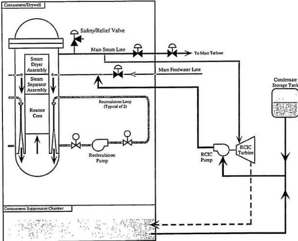
Unit 3 had a reactor core isolation cooling (RCIC) system to handle the water inventory loss associated using SRV openings to control reactor pressure. The RCIC system uses a steam-driven turbine connected to a pump to supply makeup water to the reactor vessel.
