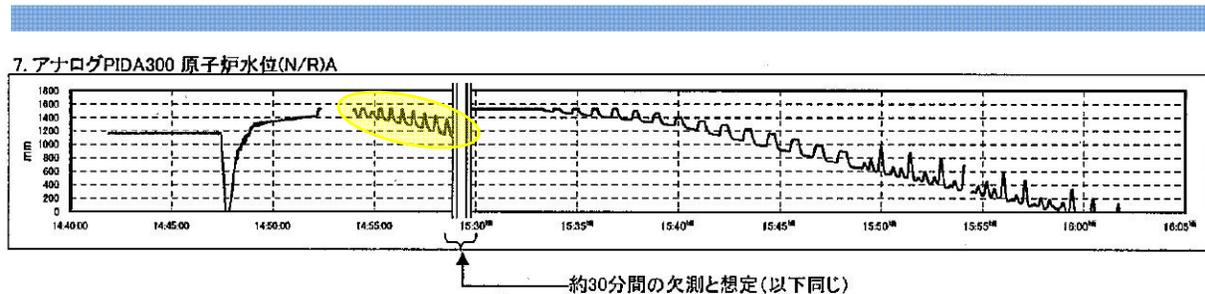
The use of SRV openings to control reactor pressure comes at the cost of losing cooling water inventory from the reactor vessel. Each time an SRV opens, water from the reactor vessel flows to the torus in the form of steam. As the chart above shows, the effect is to lower the water level inside the reactor vessel.
